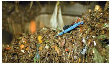
Separated contaminats consisting mainly of plastic- and carton packaging along with citrus peels coming coming out of the reject separator before going into the dewatering process. Notable is the intact "unmacerated" condition.
